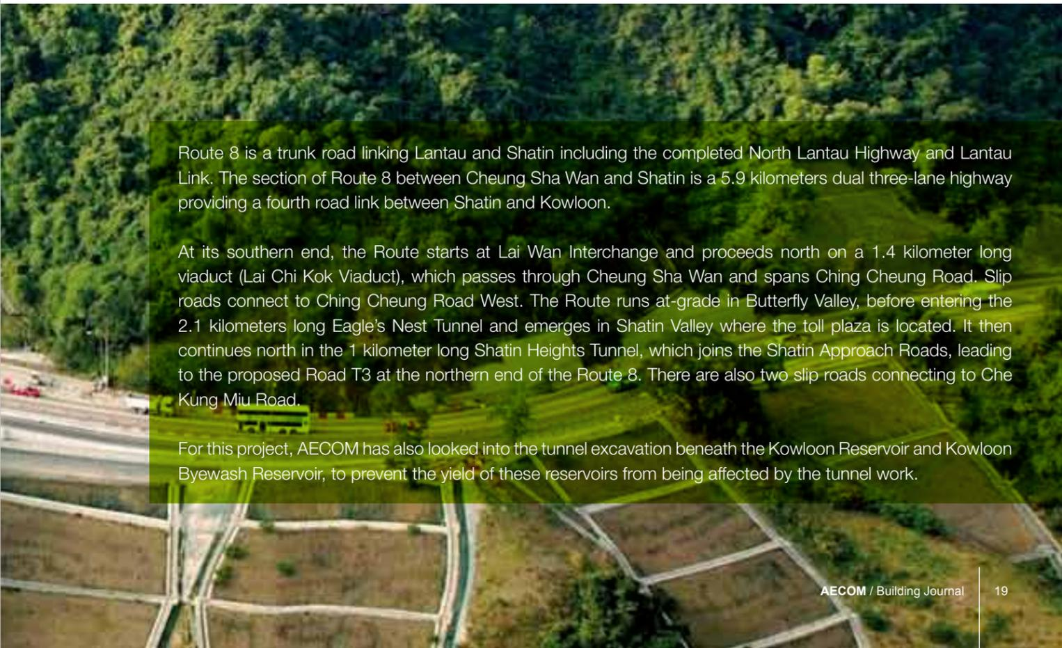
Route 8 is a trunk road linking Lantau and Shatin including the completed North Lantau Highway and Lantau Link. The section of Route 8 between Cheung Sha Wan and Shatin is a 5.9 kilometers dual three-lane highway providing a fourth road link between Shatin and Kowloon.
