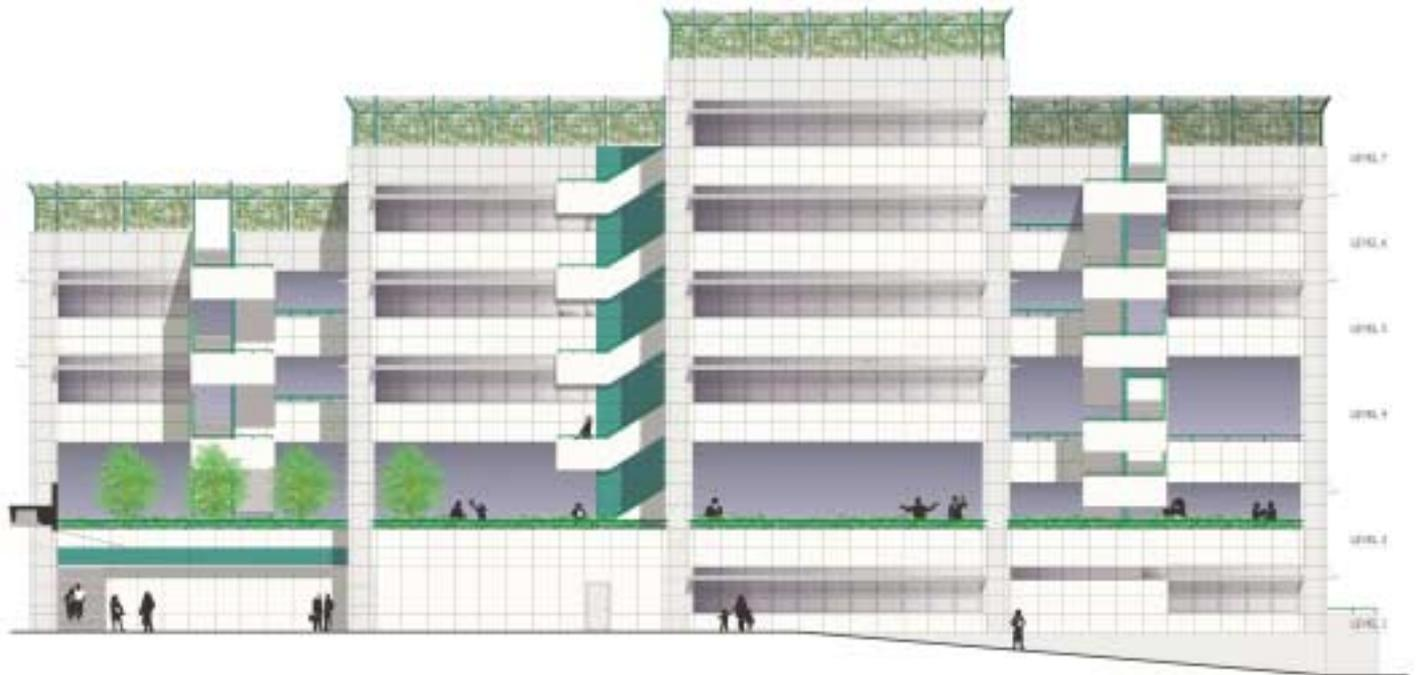
Also under the original design, the designers proposed lustre wall tiles arranged in a clearly defined grid. Time and cost considerations led to changes in materials, however, and textured spray paint was later applied instead of tiles to the exterior while retaining the grid and line detailing. Soft pastel colours are used for the four classroom wings — primary colours and the like would have looked too youthful for this project.
