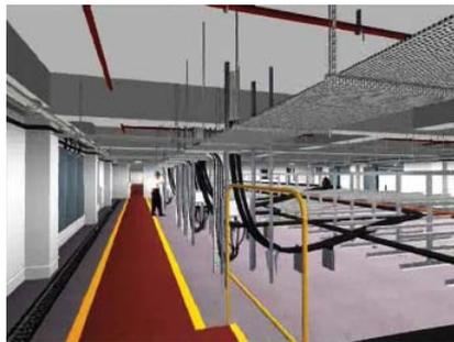
Cable basement with defined trays for power cables and demarcated escape route
