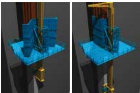
Photos 24c & 24d: Drawing showing the open and shut mold of the climb form for the mega-columns
